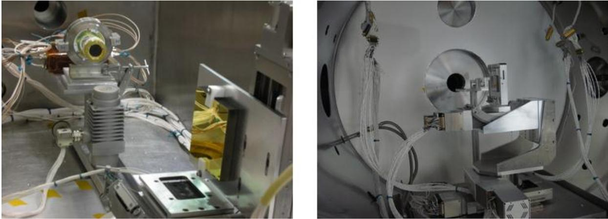
Figure 3: Left – Test grating in the University of Colorado X-ray Test Facility. Right – Test grating in the University of Iowa Facility.
