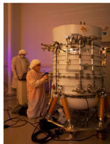
Figure 6. Assembly of the WISE payload at SDL.
