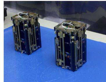
Figure 7. Two SDL-assembled DICE nano-satellites prior to launch vehicle integration
