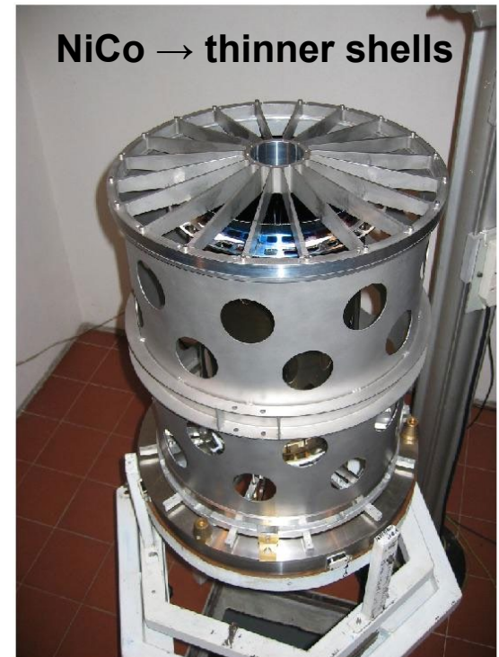
Test mirror shells installed in structure prior to testing at the MPE Panter X-ray test facility.
