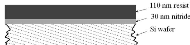
1. Spin coat resist onto nitride coated Si wafer
