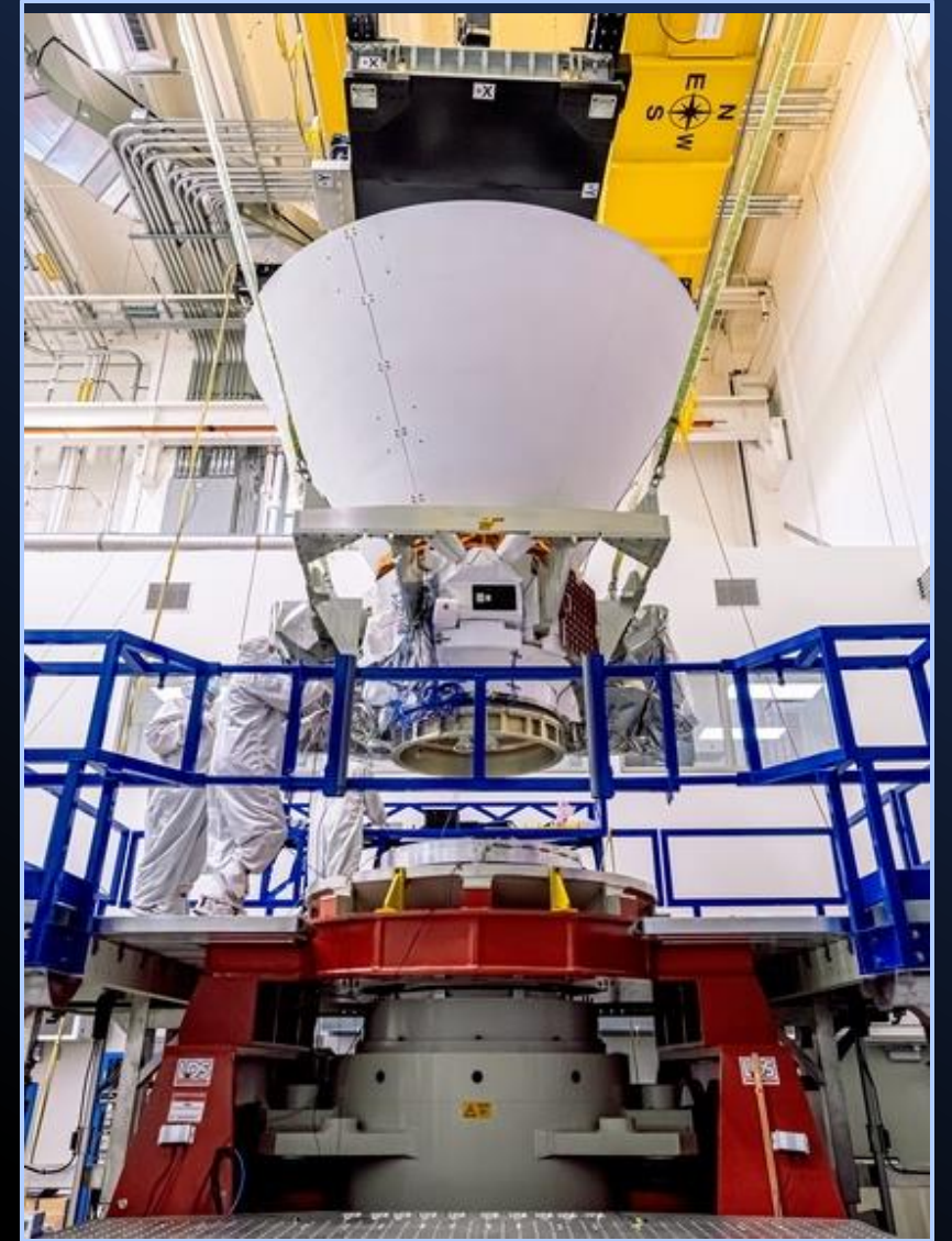
SPHEREx observatory being lifted and installed onto the vibration table, in the Z-axis configuration, at BAE Systems in Boulder CO in early August 2024.
