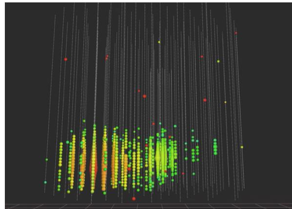
High-energy starting event view from alert IceCube-160427A. Color represents the time of the hits (red, early to green, late) and size represents detected charge. This event started in the IceCube detector volume and exited, depositing more than 100 TeV of energy. Credit: IceCube
