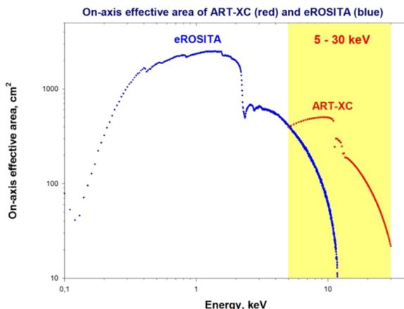
On-axis effective area of the combined 7 telescopes for eROSITA (blue) and ART-XC (red). Credit: MPE; IKI
