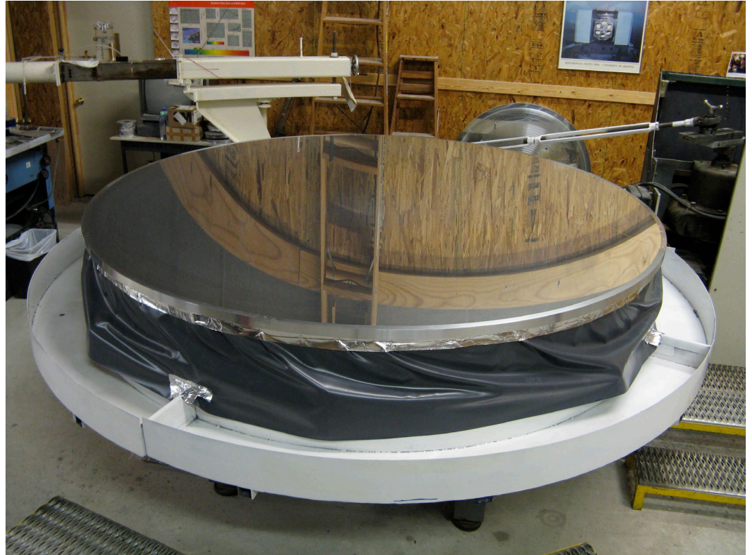
Two axis diamond turning machines 0.9 meter capacity and 2.5 meter aluminum spherical mirror on one of the two DOS large capacity polishing machines.
