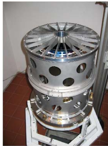
Figure 4: Telescope assembly containing two mirror shells. The angular resolution was tested at the Panter facility. The Brera Observatory and the Panter staff collaborated in the measurements.
