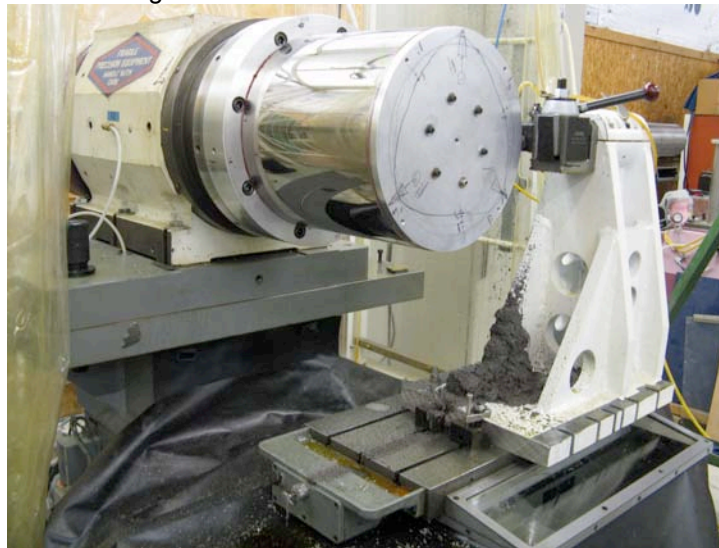
Figure 11. Single point diamond turning electroless Ni plated stainless steel slumping mandrel.
