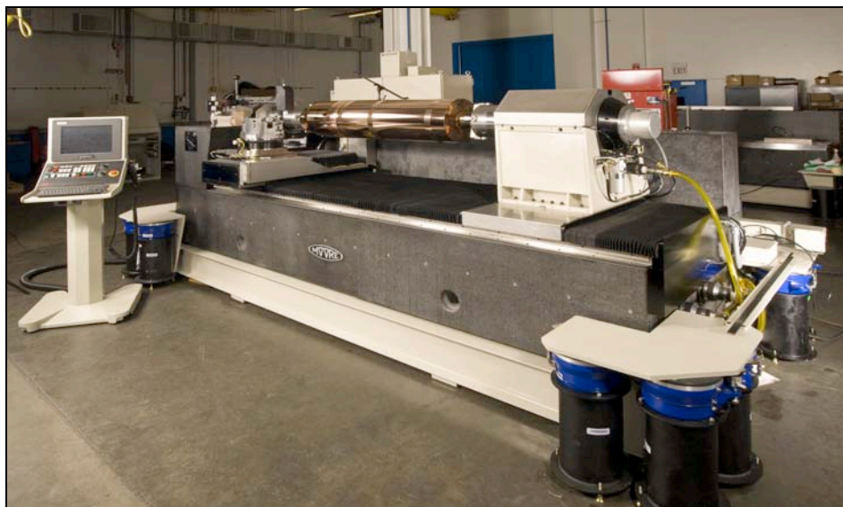
Figure 7. Large Moore granite base horizontal spindle diamond turning machine with oil hydrostatic spindle.
