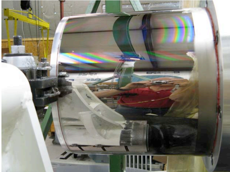
Figure 12. Electroless nickel plated 17-4PH stainless steel IXO test mandrel on a DOS diamond turning machine.
