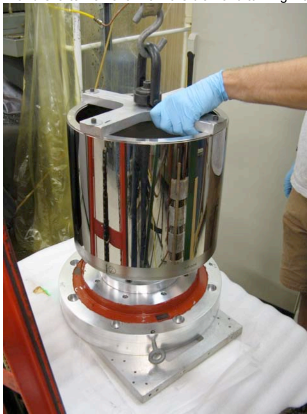
Figure 13. Diamond turned IXO test mandrel. 298mm long x 337.4mm diameter tapered cone.
