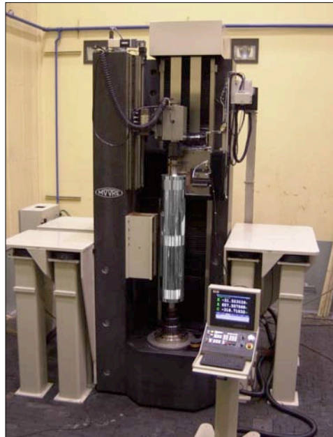
Figure 8. Large Moore vertical diamond turning machine using a vertical oil hydrostatic spindle.
