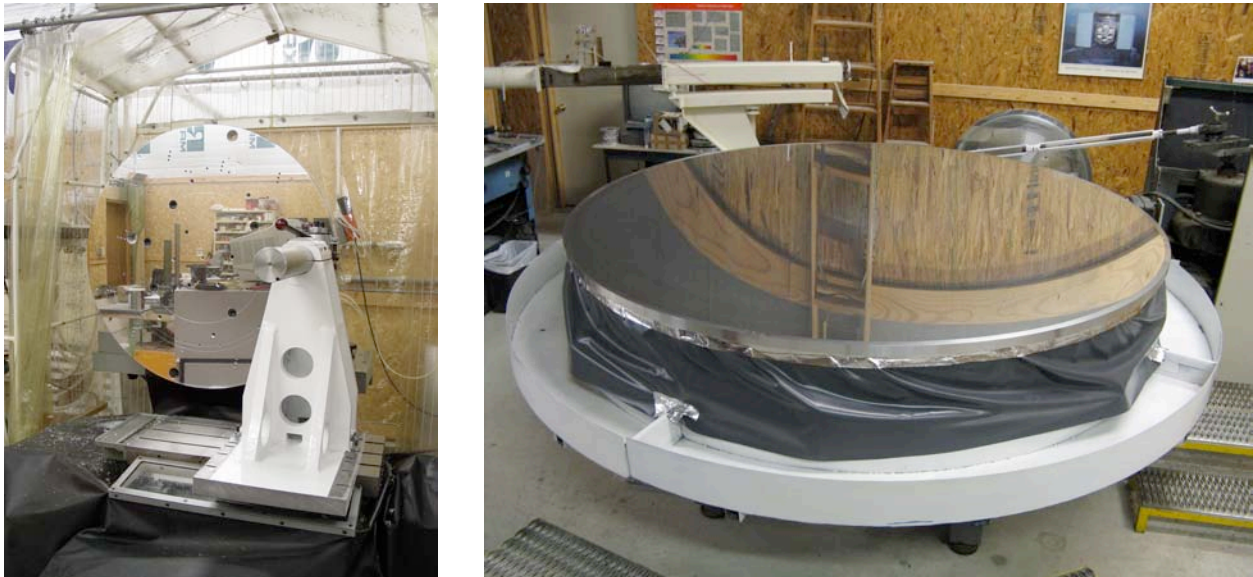
Figure 14. Two axis diamond turning machine 0.9 meter capacity and 2.5 meter aluminum spherical mirror on one of the two DOS large capacity polishing machines.
