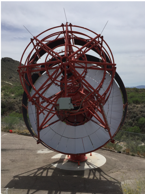
The prototype Schwarzschild-Couder Telescope (pSCT). Credit: CTA
