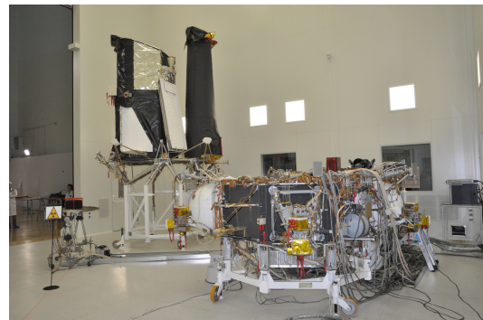
The SRG components in the NPOL assembly hall just before the first round of electrical interface tests. In the foreground, the Navigator platform. In the background, the two scientific payloads (eROSITA, left and ART-XC, right) integrated onto the mounting structure, and connected to the S/C sub-system. Credit: IKI; SRG team
